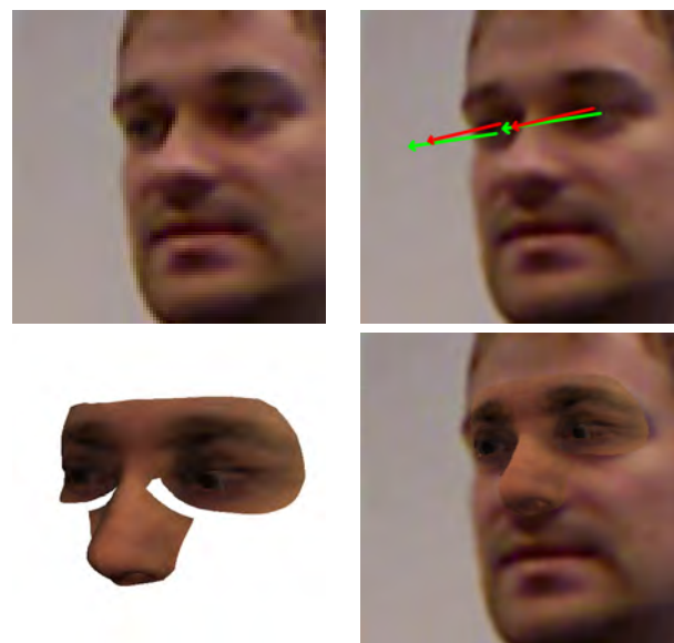
Fig. 1. Active-gaze 3DMM fitting: top left: input image; top-right: predicted gaze directions (red) and ground truth (green); bottom-left: predicted eye region model; bottom-right: eye-region model overlaid on input.
