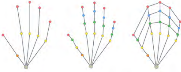
Fig. 2. Examples of different graph topologies using different sets of joints and connections. [Left] Baseline hand graph topology (11 joints - 10 connections), [Center] Hand graph topology using all hand joints (21 joints - 20 connections), and [Right] Hand topology with additional joint-level connections (21 joints - 32 connections)
