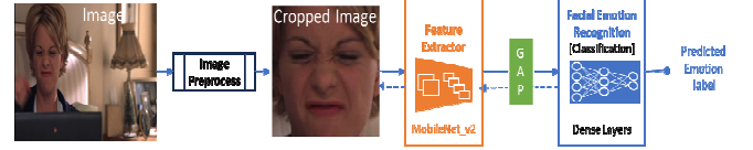
Fig 3. Image pre-processing and training pipeline for facial emotion recognition. Feature extractor is a pre-trained Mobilenet_v2 backbone which feeds into global average pooling (or GAP) layer. Finally, a set of dense layers effectively do the classification task of emotion recognition.
