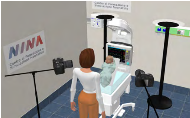
Fig. 1: Setting of data acquisition. The image shows a 3D render of the room showing the equipment used and its positioning in relation to the operator and the infant.
